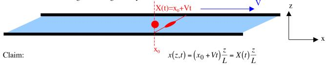
When the upper-plate velocity V is constant, the simple shear flow  $\vec{v} = v(z)\hat{x} = V\frac{z}{I}\hat{x}$  with P=0
